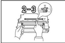
When cleaning is complete, return the *Drum Unit* to its position, aligning the guides at both ends with the slots in the printer.
